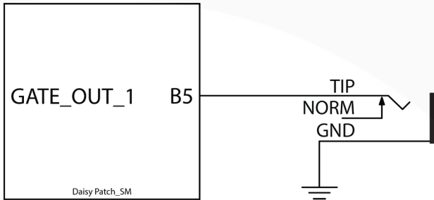
Figure 1.10 - Gate Output application example
