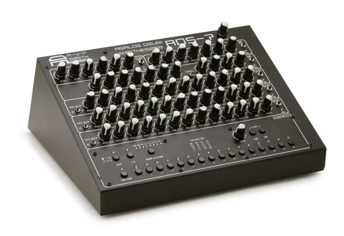
**ADS-7** - is an analog drum synthesizer inspired by the drum machines/synthesizers of the 70s-80s with a built-in 32-step sequencer and MIDI control. It has 65 controls, 4 switches and 27 buttons with which you can have a wide control over the sound parameters, sequencer and MIDI. It has individual audio outputs and individual trigger inputs for each of the seven sounds.
