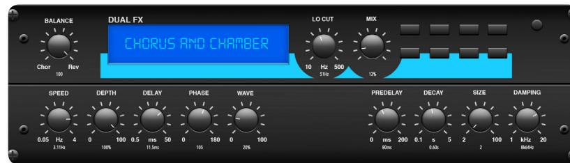
Taking up only one FX slot, the **CHORUS & CHAMBER** effect combines the shimmer and doubling characteristics of a studio-grade chorus with the sweet sound of a traditional chamber reverb. (Inspired by Lexicon PCM70\*)
