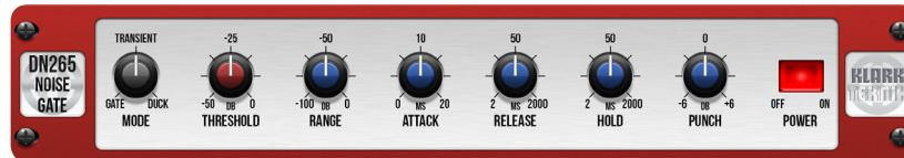
The **NOISE GATE** block sounds from passing that are below the applied threshold level, without reducing overall dynamics thanks to our proprietary Transient Accenting technology.
