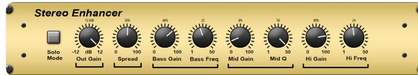
**STEREO ENHANCER** lets you emphasize the Bass, Midrange and Hi output at selectable frequencies, for maximum punch, clarity and detail – without turning up the overall volume. (Inspired by SPL Vitalizer\*)
