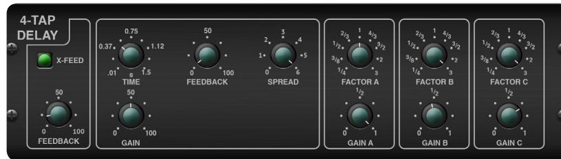
The **4-TAP DELAY** records the input signal and then echoes it back after a user-definable period of time and number of repeats. What makes the stereo and quadruple delay useful and outstanding is the linked tap-timing and musical choice of echo patterns. Use the 4-TAP DELAY to fatten up vocals and instruments, or to add an enhanced spatial element to any performance.
