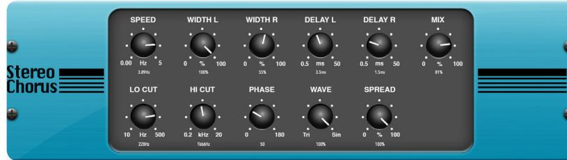
**STEREO CHORUS** samples the input, slightly detunes it and mixes it with the original signal to produce a somewhat thicker, shimmering sound. Use it to fatten up background vocals, or to double the sound of brass and woodwind instruments.
