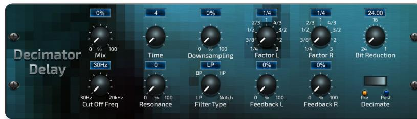
**DECIMATOR DELAY** reduces the sampling frequency and the bit-depth of the signal. The Decimator Delay is a creative tool that can be used in many ways, from emulating the aliasing noise found in older samplers, to generating complex, low-fi and rough delay lines.
