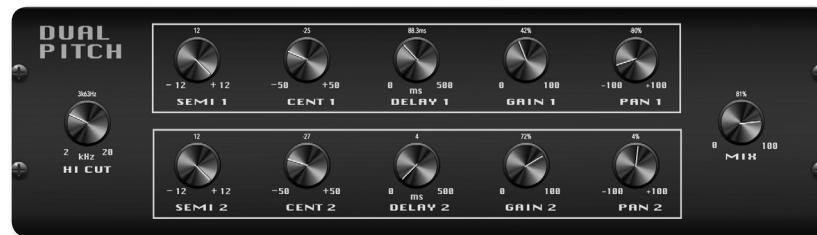
The **DUAL PITCH SHIFTER** allows you to add up to two additional notes to the original signal to create harmony. It can also be used with only a minor pitch adjustment to create much thicker sounds, often referred to as "voice doubling".
