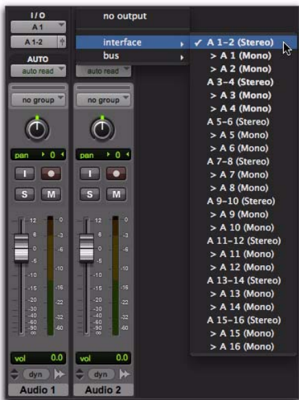
Output Path selector, Mix window
